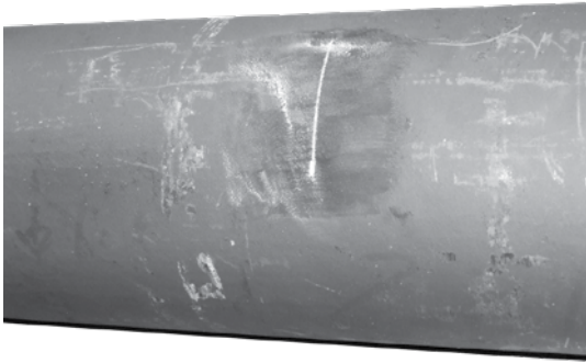
Figure 1: Previous bracket weld ground flush to axle tube surface
