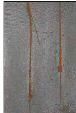
Soft coat panel after Salt Fog (ASTM B117) test: 2,000 Hours
