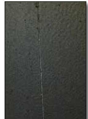
Soft coat panel after Cyclic Corrosion Testing (SAE J2334) test: 80 Cycles
