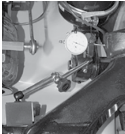
FIGURE 7-8 Check the UPPER Kingpin Bushing
