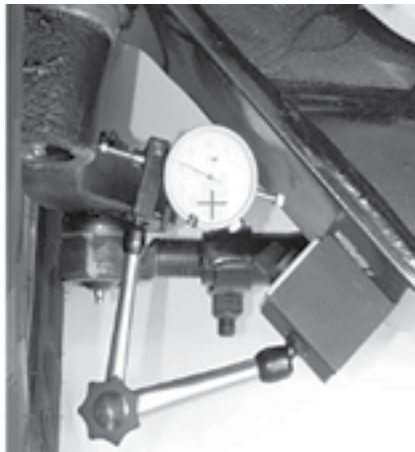
FIGURE 7-9 Check the LOWER Kingpin Bushing
