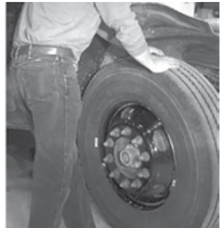
FIGURE 7-10 Move the TOP and BOTTOM of the tire in and out
