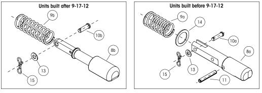
CURRENT RELEASE MECHANISMS
