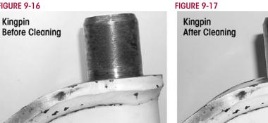
2. Inspect the kingpin for wear or damage. Use a micrometer and measure the upper and lower kingpin in two locations. Positions must be 90° opposed from each other. If the kingpin has less than 1.802" diameter, replacement of the axle is necessary, see Figures 9-18 through 9-21. Kinapin minimum dimension is 1.802".
