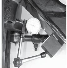
FIGURE 7-15 Move the TOP and BOTTOM of the tire in and out
