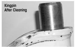
2. Inspect the kingpin for wear or damage. Use a micrometer and measure the upper and lower kingpin in two locations. Positions must be 90° opposed from each other. If the kingpin has less than 1.351" diameter, replacement of the axle is necessary, see Figures 9-18 through 9-21.
