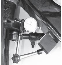
FIGURE 7-12 Move the TOP and BOTTOM of the tire in and out
