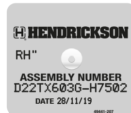
Suspension Assembly Plate – Suspension Beam
