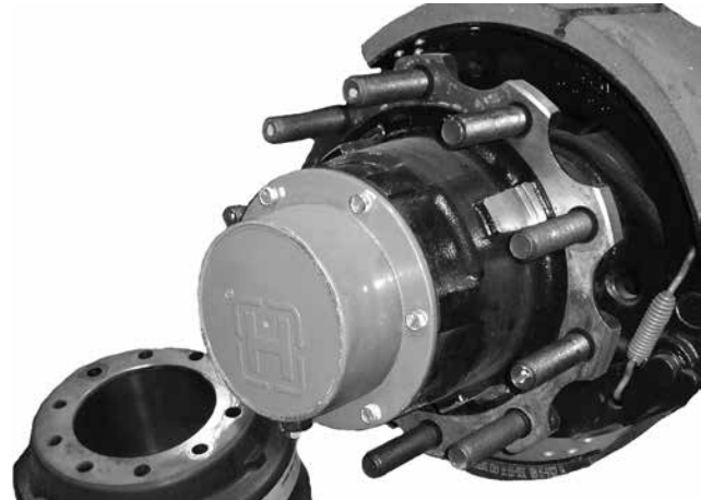
Figure 2: Brake drum removed
