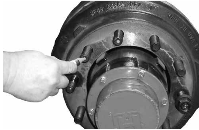
Figure 1: Identifying "old" studs
