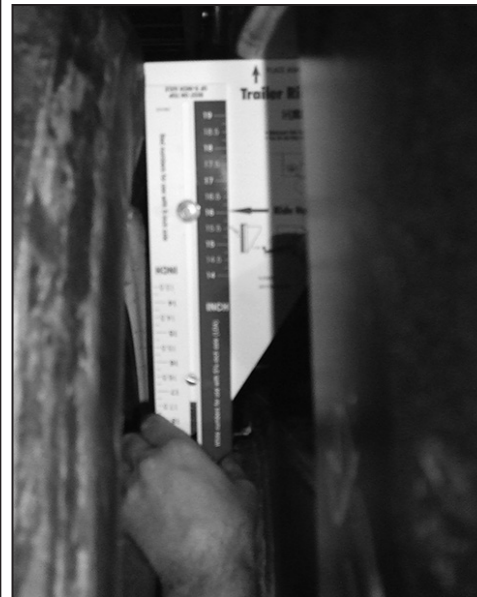
Figure 3: Using gauge to measure ride height
