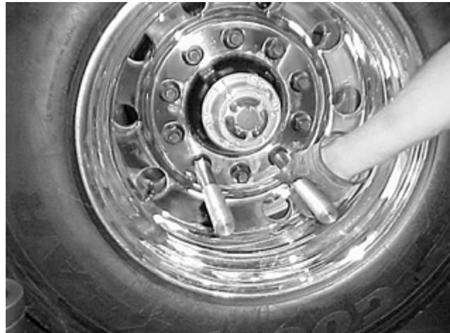
Figure 6: Installing the stud extenders
