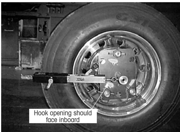
Figure 12: Attaching the extensometer to the wheel-end extender
