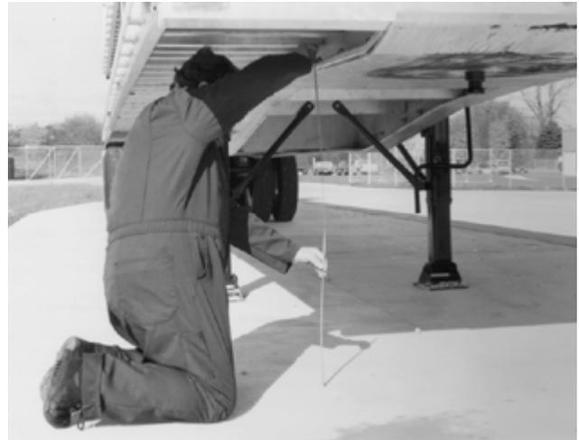
Figure 2: *Measuring kingpin height*
