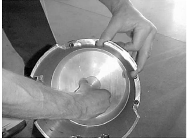
Figure 17: Checking retainer shaft for tightness
