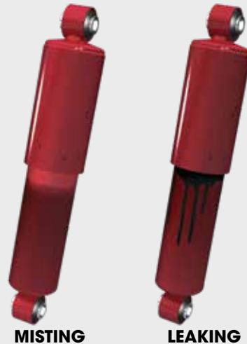
**A leaking shock absorber usually means it should be replaced, while a shock with a lightly misted outer coating can simply indicate normal operation.**
