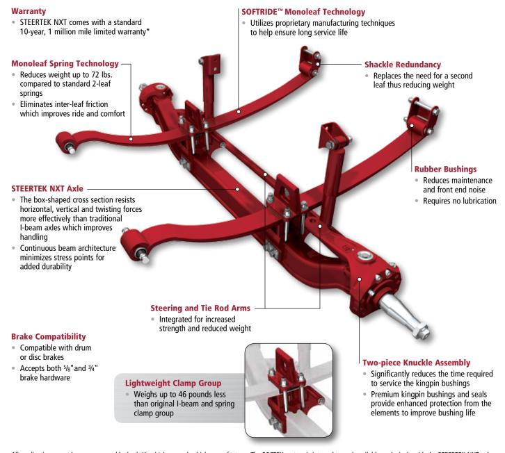
All applications must be pre-approved by both Hendrickson and vehicle manufacturer. The SOFTEK system is integral to and available exclusively with the STEERTEK NXT axle. Contact Hendrickson or vehicle manufacturer for availability.
