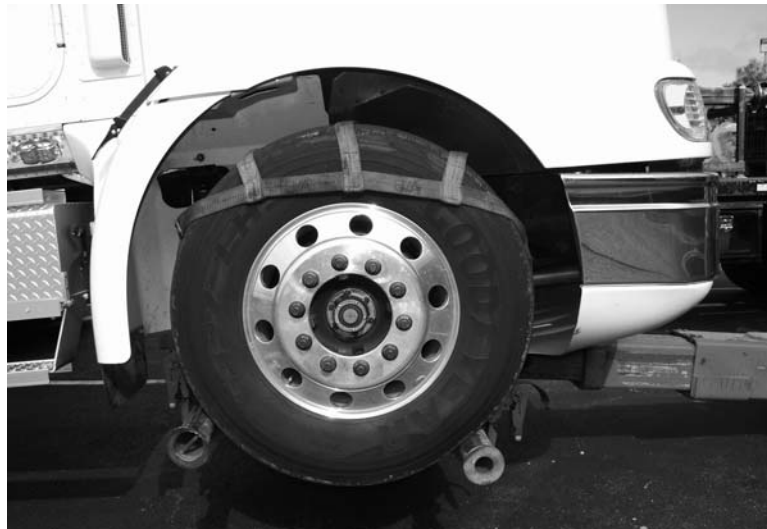
FIGURE 6-1 Wheel Lift Method
