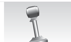
Damaged dust cover and/or shock body
