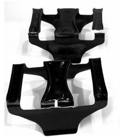
Axle Wrap Liners Unacceptable Cracks
