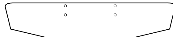
Western Star conventional. Mounting holes only. Available in stainless steel clad aluminum for Texas Square only.
