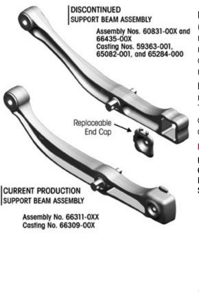
Likewise Hendrickson will only offer U-beam assembly service kits (part number 60961-XXX, see Figure 2) for any necessary replacement of PRIMAAX / FIREMAAX support beam assemblies (part numbers 66435-00X or 60831-00X) in the field. Refer to Table 1 on Page 3 to determine the U-beam assembly service kit for each respective vehicle manufacturer.
