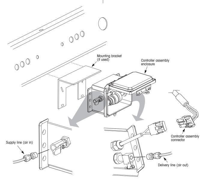
Figure 37. Controller assembly replacement
