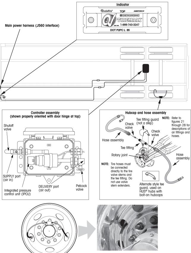
Tire hoses, with wheel guards in place on hose assemblies. Wheel guards help prevent the braided steel hoses from abrading the wheel.
