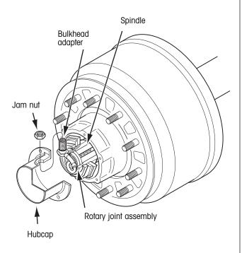
figure 39. Hubcap to bulkhead adapter removal
