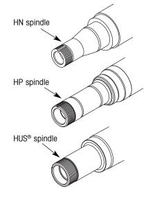
Figure 4. Axle spindle identification
