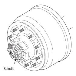
Figure 17. Completed installation of rotary joint assembly
