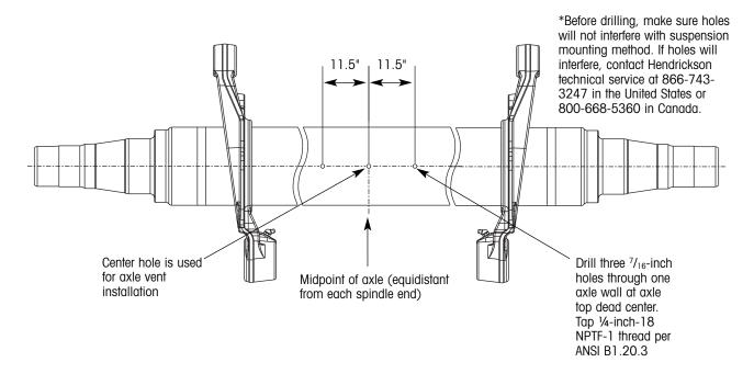
Figure 7. Hendrickson Trailer Axle drilling details
