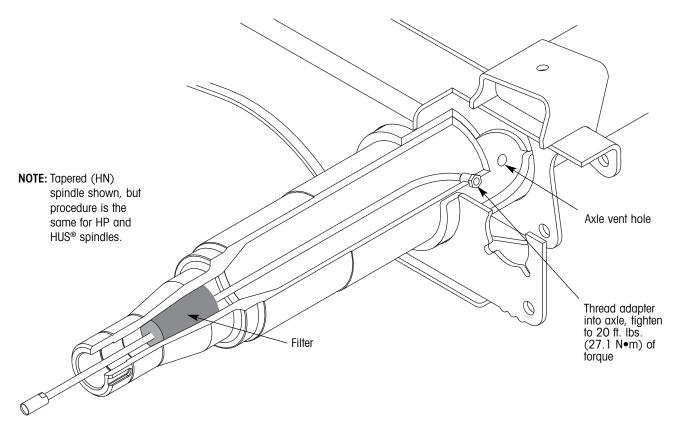
Figure 9. Installed position of hose assembly
