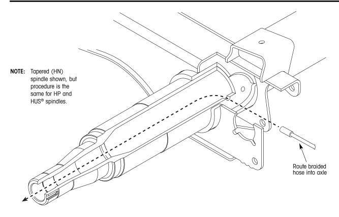
Figure 8. Routing hose in axle
