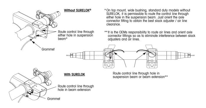
Figure 22. Suggested control line installation details for Top Mount, Wide Bushing, Standard Duty Models (AAT, HKAT)
