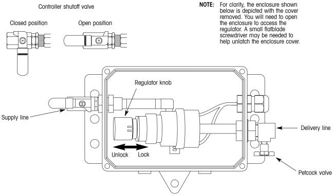
Figure 35. Setting target pressure with the IPCU
