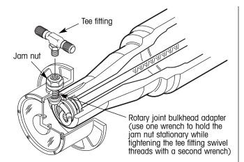
**NOTE:** A dual wheel tee fitting is shown in the illustration above, but the installation is the same for elbow-style tee fittings used on super single wheel configurations.
