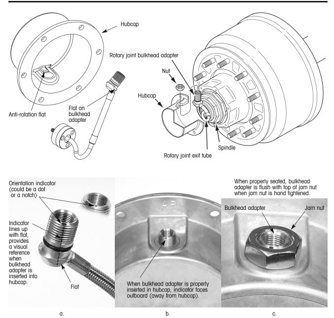
Figure 18. Hubcap to bulkhead adapter connection details
