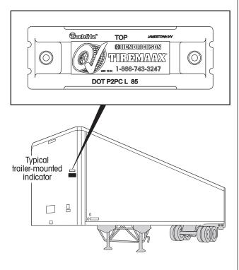
Figure 2. Trailer-mounted indicator
