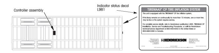
Figure 33. Recommended controller assembly mounting location and label placement
