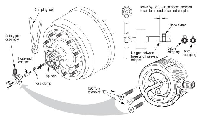
Figure 15. Rotary joint installation
