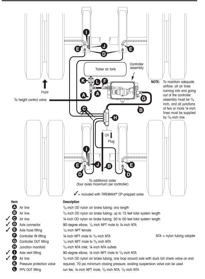
Figure 28. Typical TIREMAAX CP plumbing schematic — two axles with <sup>3</sup>/<sub>8</sub>- and <sup>1</sup>/<sub>4</sub>-inch lines and junction manifold
