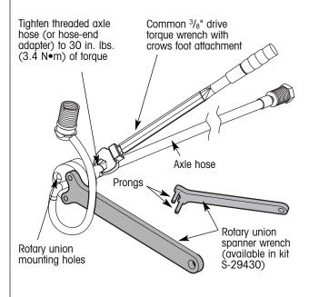
Figure 16. Rotary union spanner wrench use
