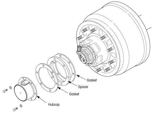
Figure 13. Hubcap spacer kit installation
