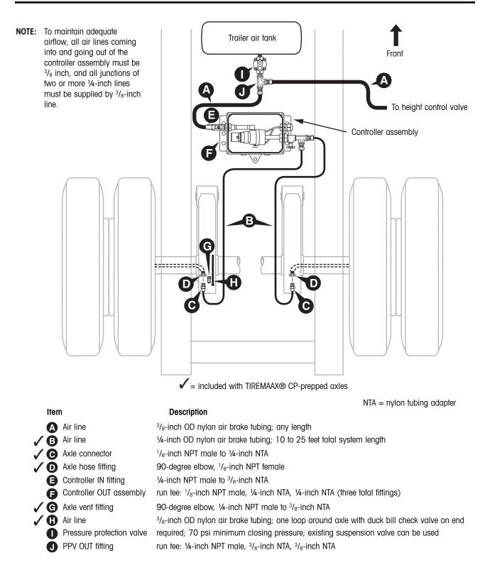
Figure 27. Typical TIREMAAX CP plumbing schematic — single axle with ¼- and ¾-inch lines
