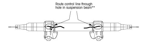
Figure 25a. Suggested control line installation details for Low Ride, Narrow Bushing, Standard Duty Models (AANL)
