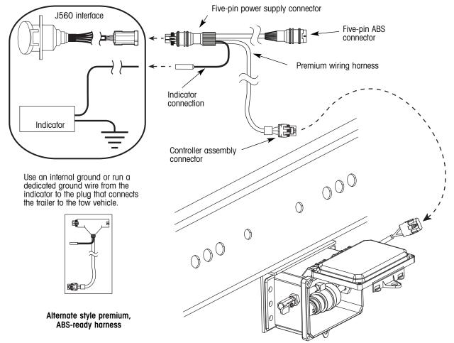
Figure 36. Premium wiring harness replacement
