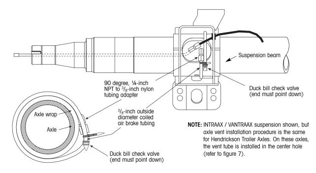
Figure 21. Typical axle vent installation
