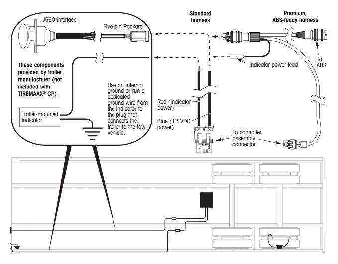
Figure 20. Trailer wiring harness installation
