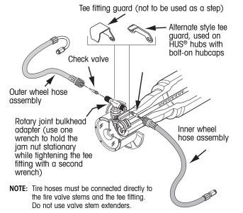
With the hubcap fitting in the 12 o'clock position, the valve stem should be located between 7 and 8 o'clock for most applications. When the wheel is installed, verify that the tire hose is not stretched so tightly that a strain is introduced at either the valve stem or hubcap fitting. Also make sure the tire hose is not so loose that it contacts the wheel.
