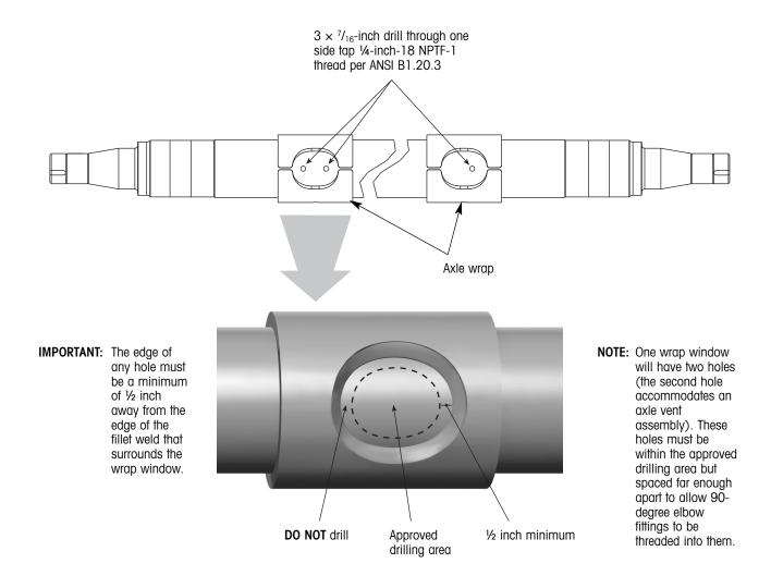
Figure 6. INTRAAX / VANTRAAX suspension axle drilling details
