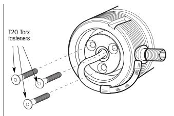
figure 40. Rotary joint removal from spindle
