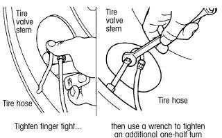
Figure 32. Attaching the tire hose to the tire valve stem
