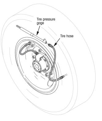
Figure 1. Manually checking tire pressure
