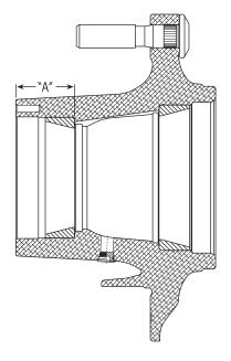
Figure 12. Minimum hub bore depth
