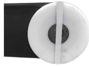
Figure 6: Bushing tube spacer installation
