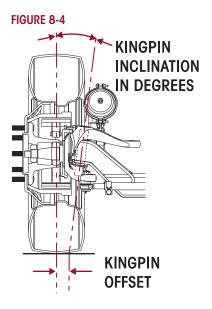
**Kingpin Inclination (KPI)** — The inward tilt of the kingpin from the vertical. This front suspension parameter has a pronounced effect on steering effort and returnability. As the front wheels are turned around an inclined kingpin, the front of the truck is lifted. This lifting of the vehicle is experienced as steering effort when the turn is executed and exhibits itself as recovery force when the steering wheel is released.
