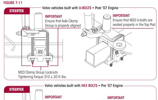
**STEERTEK:** Ensure that the bottom axle wrap is centered on the top axle wrap, see Figure 7-11.
