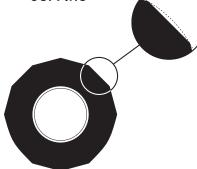
**Cupping** — Localized, dished out areas of fast wear creating a scalloped appearance around the tire. Cupping, which appears around the tire on the shoulder ribs, may also progress to adjoining ribs. See TMC RP 219A publication, page 7.
