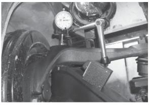
7. If vertical end play is greater than 0.030", or below 0.008" an adjustment of the upper knuckle is necessary.
