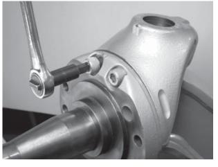
12. Remove the upper steering knuckle by sliding it up off the kingpin.
