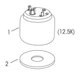
Vehicles built **between** 03/05 and 06/07, equipped with dual HCVs **must use** Air Spring with Support Plate Service Kit No. 60961-182
