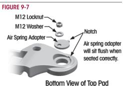
1. Insert the air spring into the top pad. Index the air spring adapter into the bottom of the top pad, see Figure 9-7. Verify that the air spring adapter notch is properly indexed into the notch in the bottom of the top pad.
