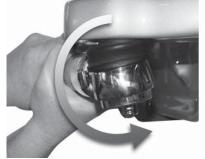
10. Position yourself directly below the tie rod end. Using both hands, grab the assembly end as close to the tie rod end as possible (no more than 6" or 152.4 mm). Apply hand pressure with reasonable human effort vertically up and down in a push-pull motion several times (using approximately 50-100 lbs. of force). Check for any movement or looseness at both tie rod end locations, see Figure 7-8.
