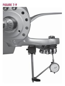
According to the Commercial Vehicle Safety Alliance (CVSA), the "out of service" criteria for front steer axle tie rod assemblies on any commercial vehicle is: Any motion other than rotational between any linkage member and its attachment point of more than <sup>1</sup>/<sub>8</sub>" (3 mm) measured with hand pressure only. (393.209(d)), (published in the North American Standard Out-of-Service Criteria Handbook, April 1, 2006.)
