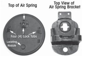
AIRING UP THE SUSPENSION SYSTEM MAKE CERTAIN THE AIR SPRING LOCATOR IS INDEXED INTO THE UPPER AIR SPRING BRACKET PROPERLY, THE LOCK TABS ARE SNAPPED INTO PLACE, AND THE AIR SPRING IS FULLY SEATED ON THE AIR SPRING BRACKET AND TOP PAD. RESULT IN PREMATURE AIR SPRING FAILURE AND CAUSE PERSONAL INJURY, OR PROPERTY DAMAGE.
