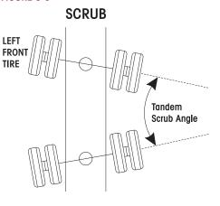
Scrub, Skew, Tram Angle or **Parallelism** — The angle formed by two thrust or tracking lines of a tandem (or multiple) axle vehicle. As indicated by the term "parallelism", the ideal condition is when the two thrust lines for a 0° angle, or are parallel to each other. Positive skew or tram is when the distance between the right axle ends is less than the distance between the left.
