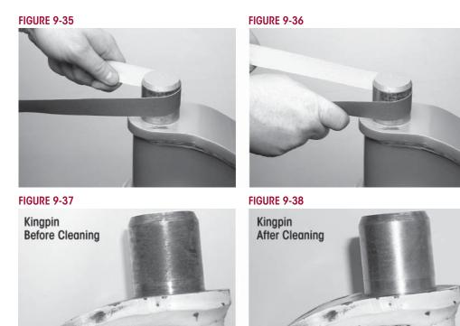
2. Inspect the kingpin for wear or damage. Use a micrometer and measure the upper and lower kingpin in two locations. Positions must be 90° opposed from each other. If the kingpin has less than 1.802" diameter, replacement of the axle is necessary, see Figures 9-39 through 9-42.
