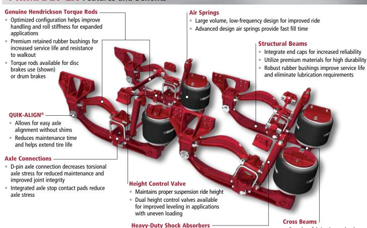
Positioned and tuned for optimum damping characteristics
