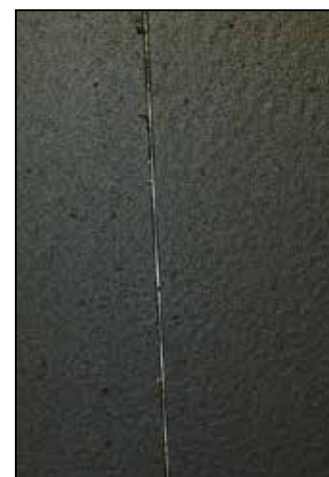
Soft coat panel after Cyclic Corrosion Testing (SAE J2334) test: 80 Cycles
